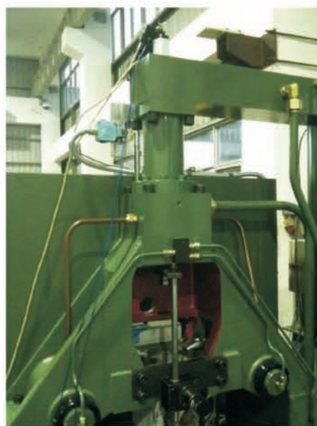
Hot chamber die-cast machine used Germanjet 17 series
